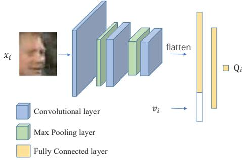
Figure 3. The architecture of frame evaluation network. The kernel sizes of convolution layers are  $9 \times 9$ ,  $4 \times 4$  and  $3 \times 3$ , respectively. Both the max pooling layers have kernel size  $2 \times 2$  and stride 2. The feature dimension of the first two fully connected layers are set as 64. All hidden layers use PReLU [13] as the activation functions.
