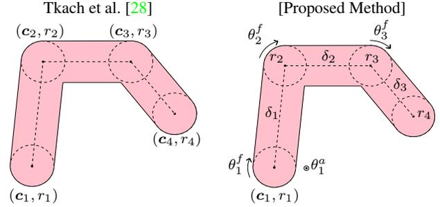
Figure 7: Sphere-mesh vs. our  $[\theta, \beta]$  parameterization.
