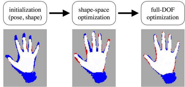
Figure 3: In initialization our calibration algorithm receives the default template tracked by [28] that provides an initialization of pose and shape. We then optimize for a coarse shape in a low-dimensional shape-space, and finally perform a local refinement in the full-dimensional domain.
