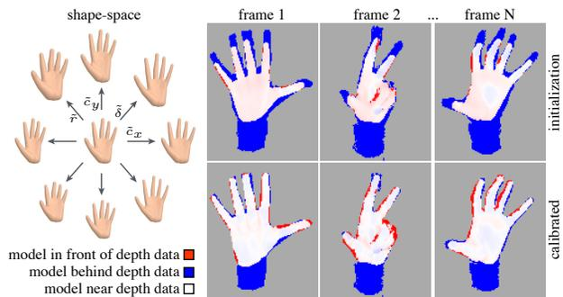
Figure 1: Our low-dimensional latent space directly encodes shape variations as local anisotropic scalings of a template model. (left) A visualization of the shape-space, encoding palm/finger length compression/stretching and sphere-mesh radii. (right) Calibrating in the reduced shape-space followed by a fine scale refinement leads to a robust calibration algorithm – remaining errors are largely due to sensor artefacts.
