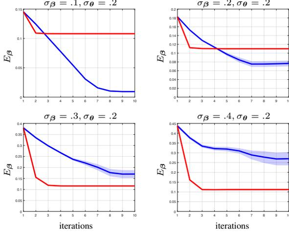
Figure 8: A comparison of the convergence properties of the re-parameterized **full-DOF** (112 parameters) vs. **reduced-DOF** (5 parameters) calibration. As we increase the perturbation, the full-DOF optimization loses robustness as illustrated by the variance plots. Conversely, the reduced-DOF optimization is highly robust, although it only provides a rough approximation of the parameters.
