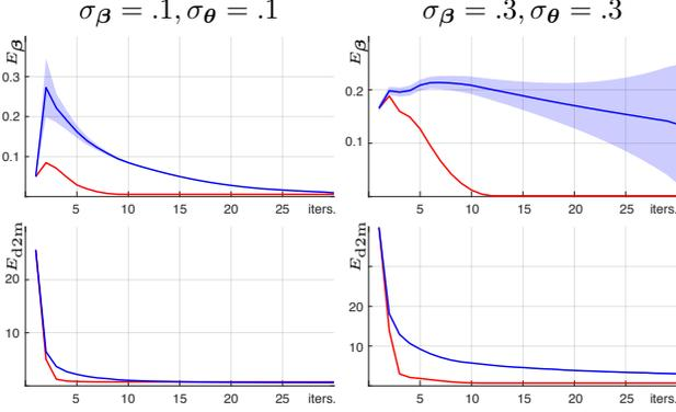
Figure 5: In this test, we calibrate a single finger and show how the convergence properties improve switching from a **position-based** [28] to our **decoupled**  $[\theta_n, \beta]$  formulation. The shading denotes one standard deviation  $\sigma$  of uncertainty; note that although variance is always plotted, at times it is not visible (i.e.  $\sigma \approx 0$ ).  $E_\beta$  and  $E_{d2m}$  are respectively defined in Eq. 13 and [28].
