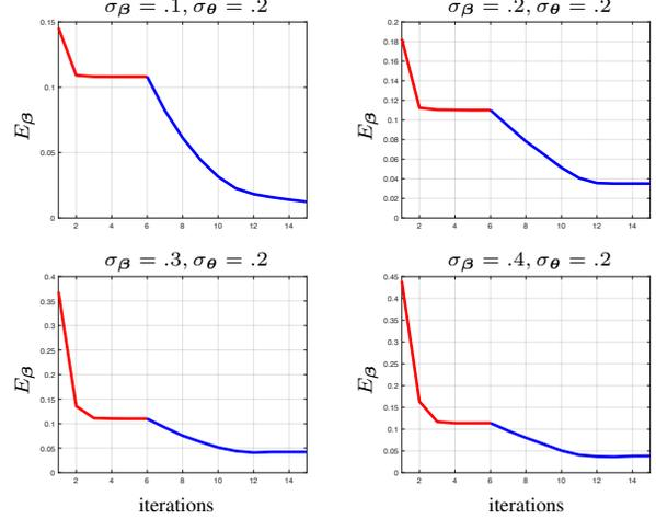
Figure 9: The 2-stage algorithm outlined in Figure 3 combines the robustness of the **reduced-DOF** to the accuracy of the **full-DOF** calibration. For visualization purposes only, we execute five iterations of reduced-DOF optimization; note in all our experiments, five iterations are sufficient to achieve convergence of the low-dimensional solve. Note how variance  $\approx 0$ , revealing enhanced convexity.
