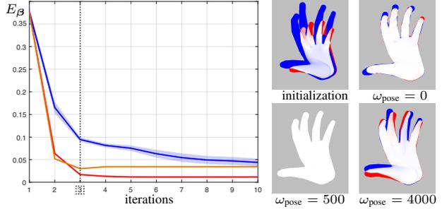
Figure 4: The decoupled parameterization allows to damp updates in pose and shape with different weights, leading to faster and more robust convergence. (left) In the plot above we analyze the convergence for  $\omega_{\text{pose}} = \{0, 500, 4000\}$ . (right) We illustrate the calibrated model at iteration 3.
