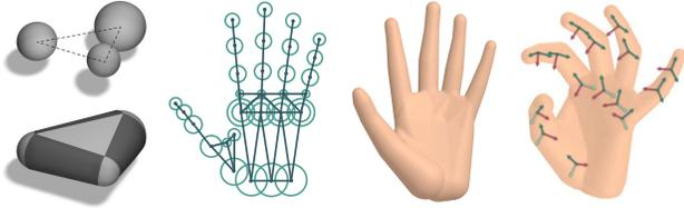
Figure 2: (a) A basic sphere-mesh component whose surface is the convex hull of spheres whose radii are defined on the skeleton vertices. (b) The sphere-mesh hand topology and (c) the rest-pose tracking template. (d) The posed template, and a visualization of the kinematic frames  $\{\mathbf{T}_k\}$ .
