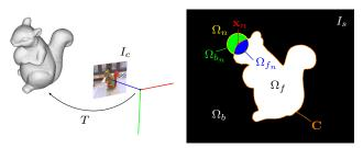
Figure 2. Overview of our pose estimation setting. Left: The object pose T relative to a camera based on color image  $I_c$  and a 3D model of the object. Right: Silhouette  $I_s$  generated by projecting the surface model into the image plane using an estimated pose T.
