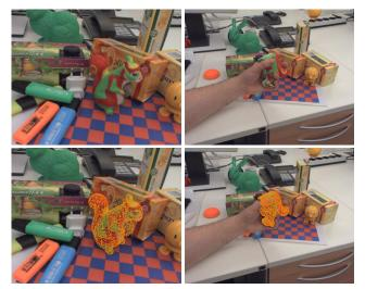
Figure 1. Estimating the pose of a heterogenous object in a cluttered scene under strong occlusions and viewpoint changes. Top: RGB input frames. Bottom: Tracking result (within  $\sim 16$  ms).
