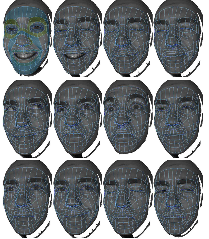
Figure 6: 3D surface tracking for facial surfaces with large expression changes.
