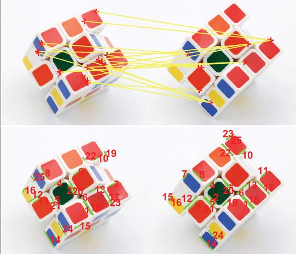
Figure 1. Plenoptic SfM (P-SfM) using point vs. line features. Top: Regular SIFT point feature matching produces insufficient inliers, Bottom: Our technique produces sufficient line matching for reliable P-SfM with 16 inliers out of 25 matches.
