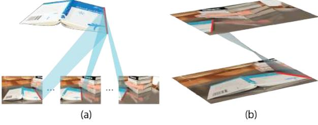
Figure 2. Line-ray manifold. A 3D line projects to 2D lines in individual images (a) but maps to a bilinear surface in a 3D LF (b).
