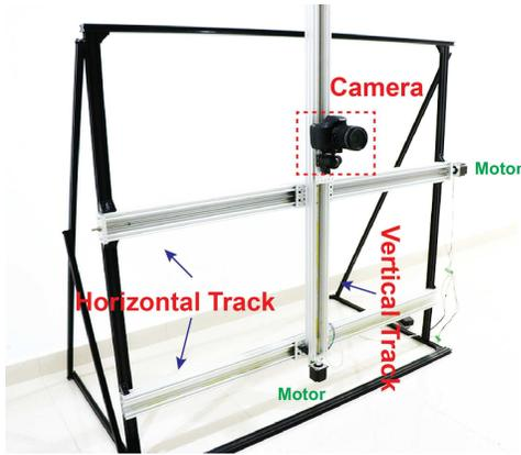
Figure 5. Our camera array that can capture  $7 \times 7$  large scale LFs. We mount a pre-calibrated Canon 760D camera on an electrically controlled rig.
