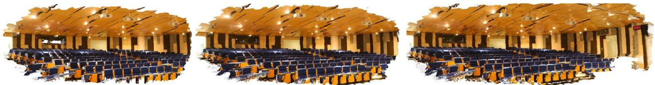
Figure 9. Our P-SfM results on large scale scenes. We captured LFs using a camera array at 3 different positions, we estimate poses of the LFs, and show the fused stereo results. From left to right: single point cloud, fused two point clouds and fused three point clouds.
