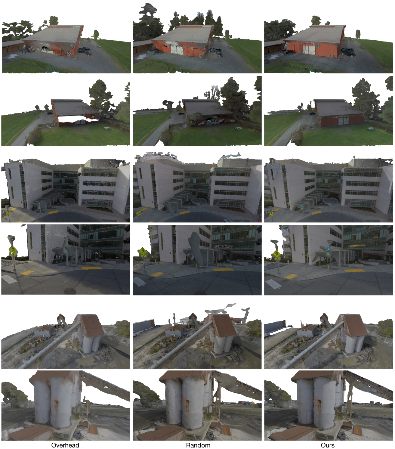
Figure 2. Qualitative comparison of the 3D reconstructions produced by overhead, random, and our trajectories for three real-world scenes. Our reconstructions contain noticeably fewer artifacts than the baseline reconstructions. In all our experiments, we control for the flight time, battery consumption, number of images, and quality settings used in the 3D reconstruction. Best viewed digitally at high resolution.
