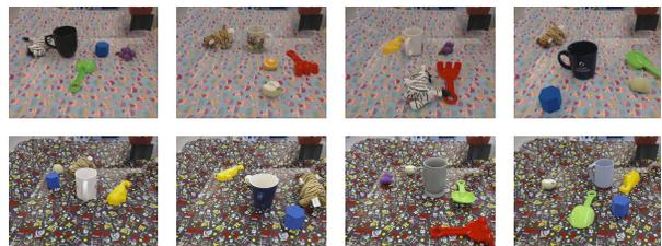
Figure 3. A sample of the test environments for the real robot experiments. Note that the mug being manipulated, the background, and the distractor objects were all unseen during training - in both the expert demonstration and weakly labeled images.
