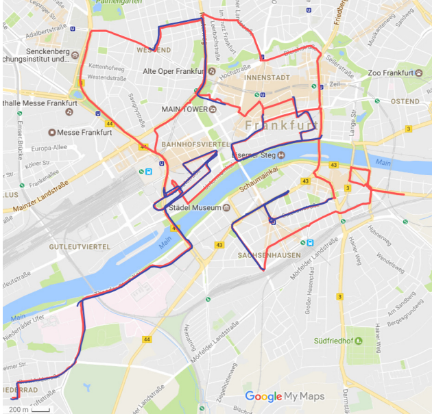
Figure 2: The full Frankfurt trajectory superimposed on the corresponding Google Map scene. The trajectory estimates of the subsections (blue) are aligned to the ground truth trajectory (orange) using a rigid-body transformation (6DoF). Best viewed printed.
