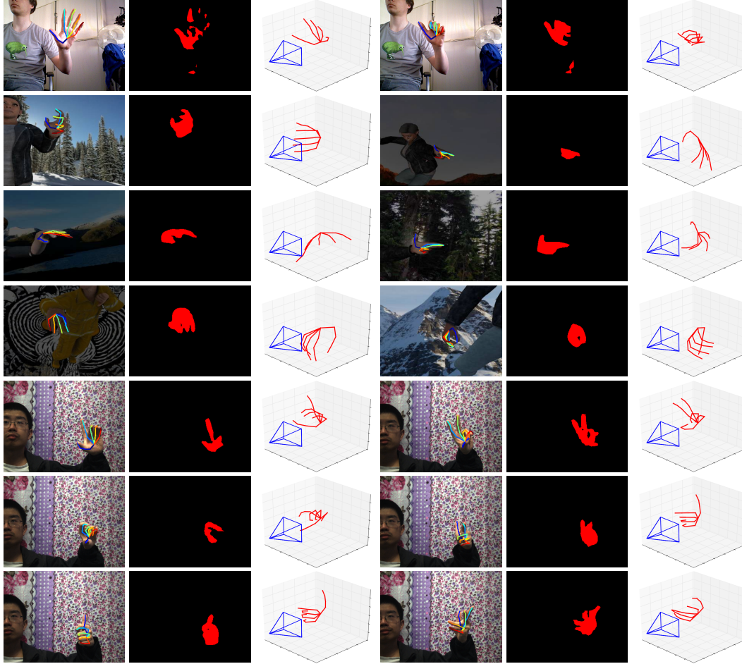
Figure 1: Qualitative examples of our complete system. Input to the network are color image and information if its a left or right hand. The network estimates the hand segmentation mask, localizes keypoints in 2D (shown overlayed with the input image) and outputs the most likely 3D pose. The top row shows samples from a dataset we recorded for qualitative evaluation, the following three rows are from R-val and last three rows are from S-val .
