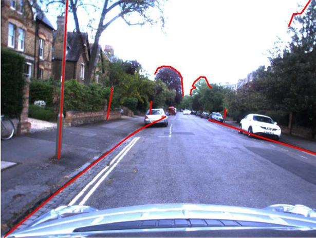
Figure 4. An image from the mapping sequence, together with the reprojections of the 3D curves in the model.
