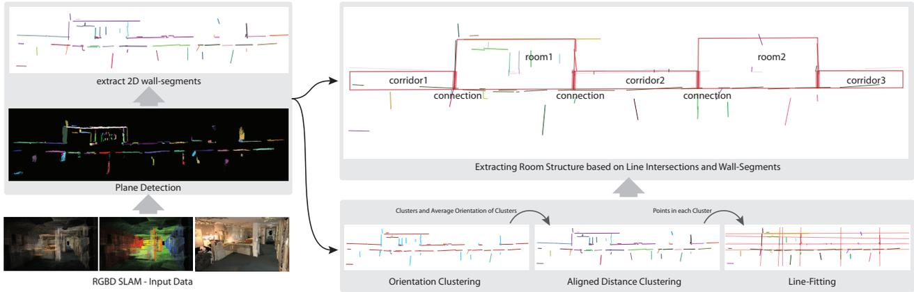
Figure 5: Extracting Floor-Plan Semantics from 3D SLAM Data
