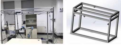
Figure 4. The left is overlook about our robotic system. The right shows the position and observation of the four cameras
