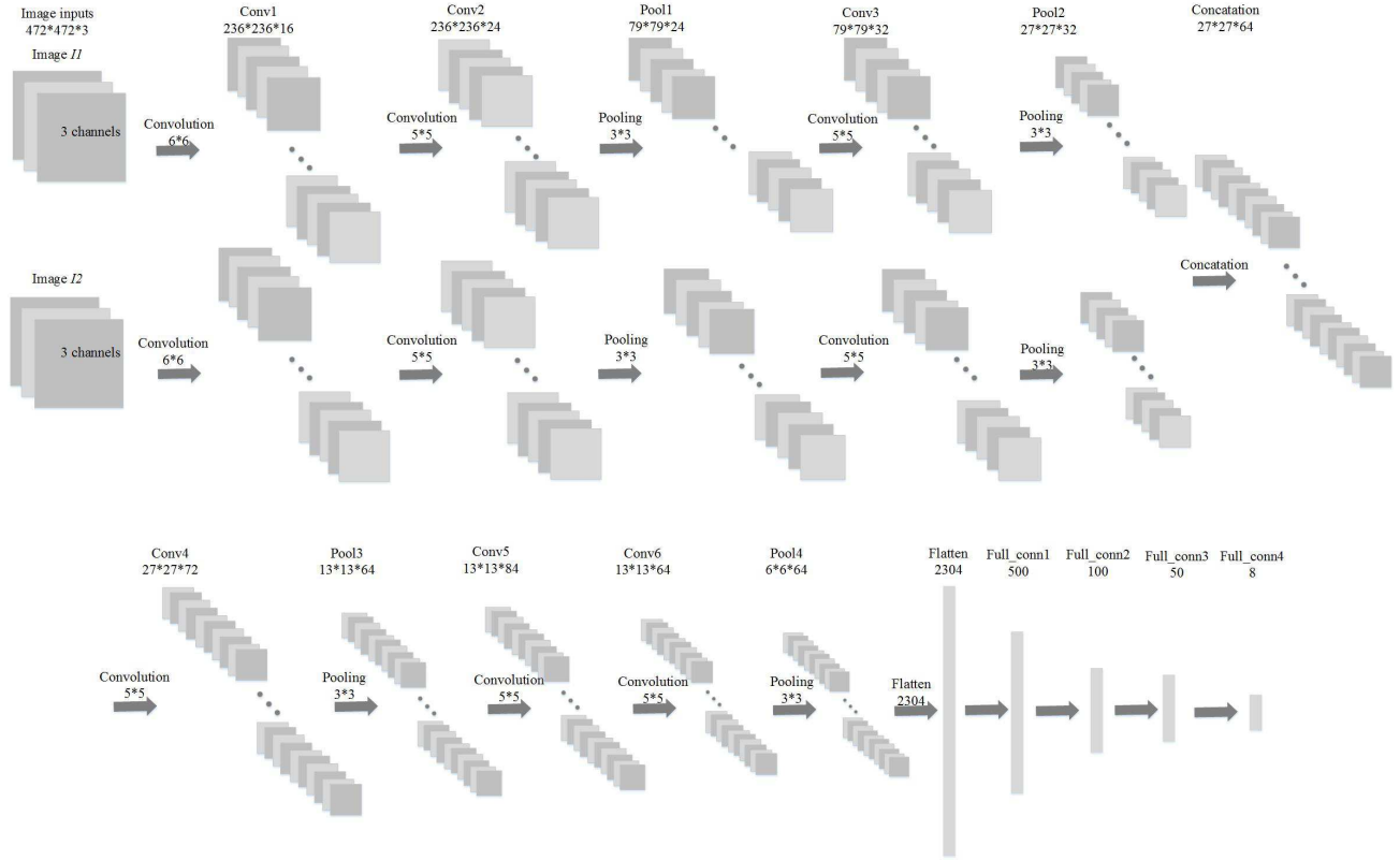
Figure 8: The architecture for the Deep Convolutional Neural Network used in our method. The input image I_1 , as well as image I_2 , are all fed into a 6 \times 6 convolution with stride 2, followed by a 5 \times 5 convolution and a 3 \times 3 max-pooling. This is followed by a 5 \times 5 convolution and a 3 \times 3 max-pooling again. Then they are merged to the size of 27 \times 27 \times 64 using concatenation. The result is then processed by three 5 \times 5 convolutions, two 3 \times 3 max-pooling layers, and four fully connected layers after which the network outputs the classification result.
