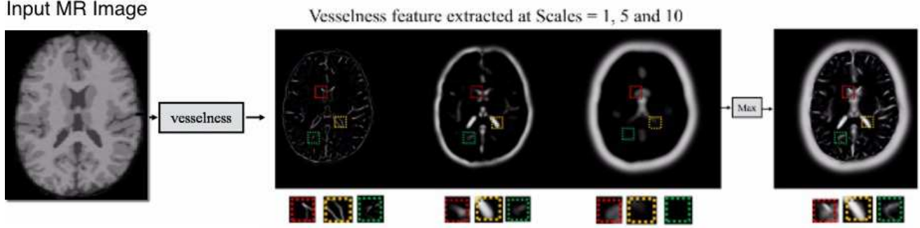
Figure 2. Demonstrates the pipeline of vesselness features at 3 scales. For each feature map extracted at each scale, a 20 \times 20 patch is selected. Here only 3 scales are shown as opposed to 10 used in our experiments owing to space restrictions. Finally, Max operation is performed across scales to achieve scale invariance.
