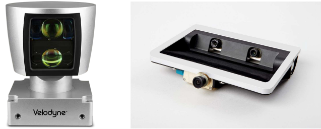
Figure 2: Lidars and cameras are the main sensors used to map the road ahead of the car. Left: Velodyne HDL-64E lidar, which costs ca. $75,000. Right: Volvo's customized windshield camera array. Sources: Velodyne and Volvo.
