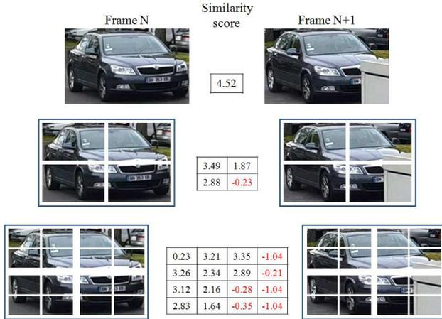
Figure 2: Occlusion detection using quad-tree decomposition.
