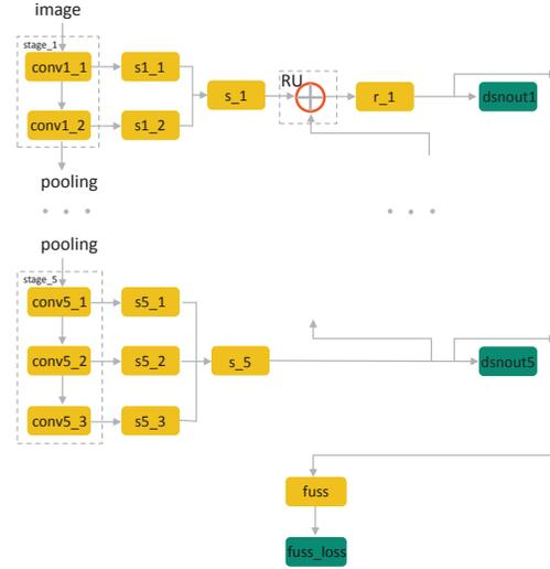
Figure 2. The base architecture integrating RCF and SRN.
