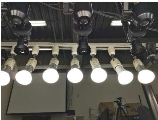
Figure 6. Multiple RGB cameras. Three high-resolution cameras are installed to acquire the dense 3D structure of leaves from the top.
