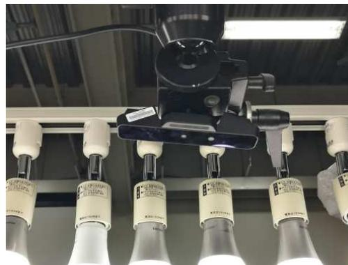
Figure 5. RGB-D camera. Intel RealSense SR300 is selected because it is optimized for capturing an object at a short distance such as 20-150 cm.
