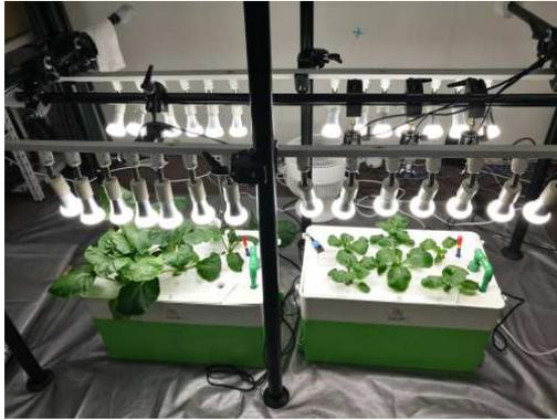
Figure 1. Platform to create KOMATSUNA datasets in indoor environments. To cultivate plants, a compact and complete platform for 3D plant phenotyping was developed using commercial devices only.
