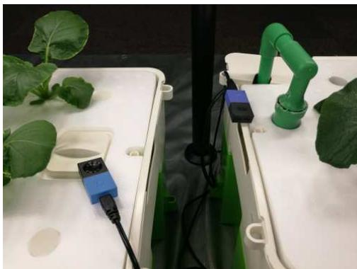
Figure 4. Sony MESH (two color boxes at the center of the image). Ambient temperature, humidity and brightness can be measured. The unit of brightness is in lux. The data is transferred to a smart-phone using Bluetooth.
