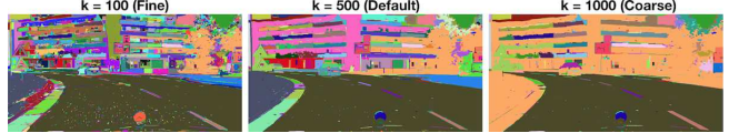
Figure 3. Graph-based superpixels [11]. The threshold parameter k decides how coarsely the image will be segmented by the superpixels.
