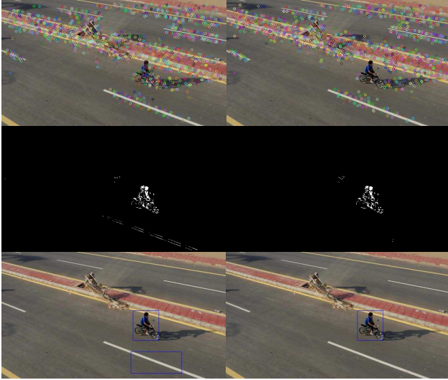
Figure 2. Effect of filtering keypoints on moving objects (from previous detection) before calculating the current homography matrix. Top to bottom; extracted keypoints, thresholded two frame difference and final results are given. Left and right column images show the results without and with the proposed keypoint filtering loop, respectively.
