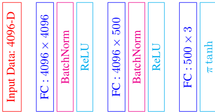
Figure 2: Pose Network for the axis-angle representation
