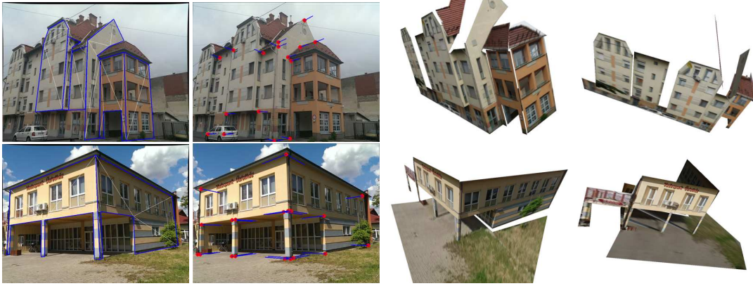
Figure 5: Reconstruction of real buildings. From left to right: selected regions in first image; regions with reconstructed normals; two different views of the reconstructed and textured 3D scene.
