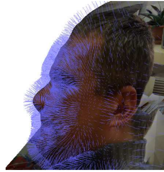
Figure 7: Reconstructed 3D face with surface normals colored by blue.
