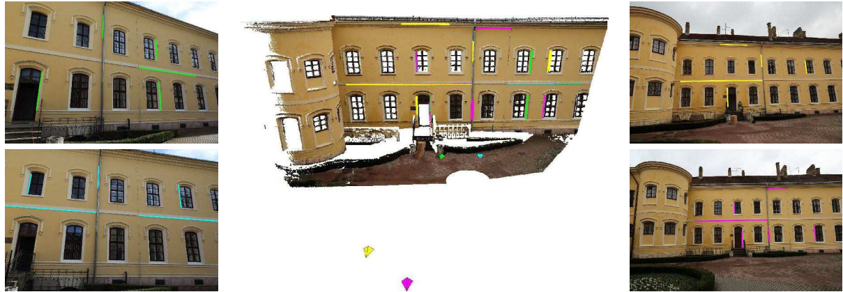
Figure 7: Lidar laser scan for testing our pose estimation algorithms with 4-camera system. 2D detected lines are shown next to the 3D point cloud which colors are the same to their corresponding camera.
