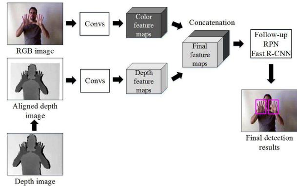
Figure 2. Hand detection pipeline of two-streams Faster R-CNN.
