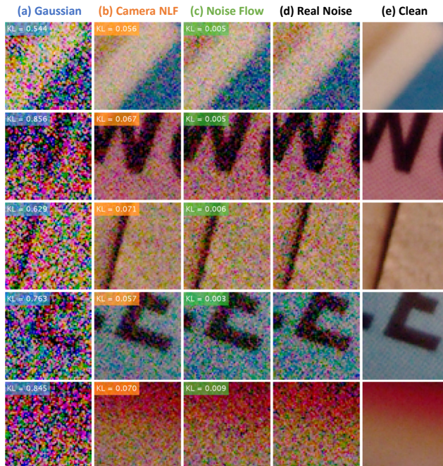
Figure 1: Synthetic noisy images generated by (a) a Gaussian model, (b) a heteroscedastic signal-dependent model represented by camera noise level functions (NLF), and (c) our Noise Flow model. Synthetic noise generated from Noise Flow is consistently the most similar to the real noise in (d), qualitatively and quantitatively (in terms of KL divergence relative to the real noise, shown on each image). (e) Reference clean image. Images are from the SIDD [1].
