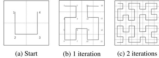
Figure 3: The construction of Hilbert curves.
