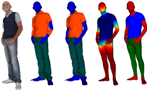
Figure 4: Left to right: Scan, segmentation with MRF and CNN unaries, MRF with CNN unaries + garment prior + appearance terms, the garment(t-shirt) prior based on geodesics and the template. Notice how the garment prior is crucial to obtain robust results.
