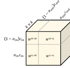
(b) The Octave Convolution kernel. The  $k \times k$  Octave Convolution kernel  $W \in \mathbb{R}^{c_{in} \times c_{out} \times k \times k}$  is equivalent to the vanilla convolution kernel in the sense that the two have the exact same number of parameters.
