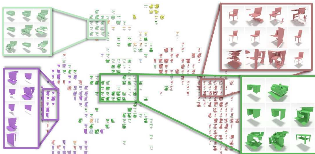
Figure 1: We learn a joint embedding space of scan and CAD object geometry, visualized here by t-SNE. Semantically similar objects lie close together, despite very different lower-level geometric characteristics (clutter, noise, partialness, etc).
