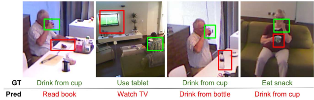
Figure 5. Separable STA correctly discriminates the activities with fine-grained details. The model without attention (I3D) is misled by imposter objects (displayed in red boxes) in the image whereas our proposed separable STA manages to focus on the objects of interest (displayed in green boxes).
