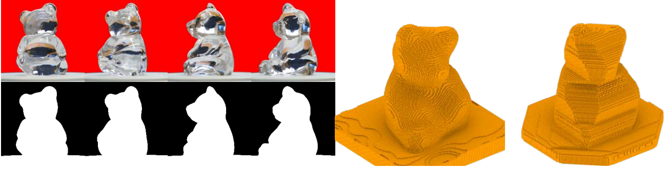
Figure 6: Shape-from-silhouette reconstruction using captured images. For this glass object, we photographed 4 views, with 45^\circ angle apart, against a uniform background color. We then applied background-color removal and converted each image to binary silhouette image. The first reconstructed model is the result using our deep prior, whereas the second is the result using the space carving baseline.
