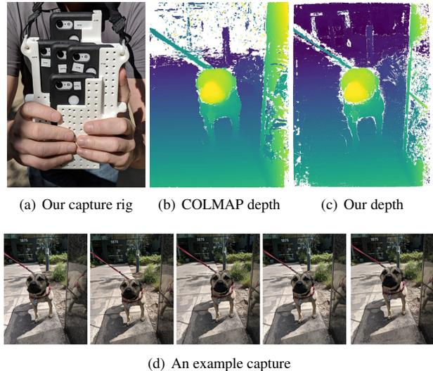
Figure 4. Our portable capture rig with synchronized cameras (a) can be used to capture natural in-the-wild photos, where each central image is accompanied with 4 additional views (d). These multiple views allow us to use multi-view stereo algorithms to compute “ground truth” depths and confidences, as shown in (b) and (c) (low confidence depths are rendered as white).
