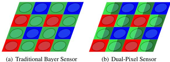
Figure 2. A modern Bayer sensor consists of interleaved red, green, and blue pixels underneath a microlens array. (a). In dual-pixel sensors, the green pixel under each microlens is split in half (b), resulting in two green images that act as a narrow-baseline stereo camera, much like a reduced light field camera.
