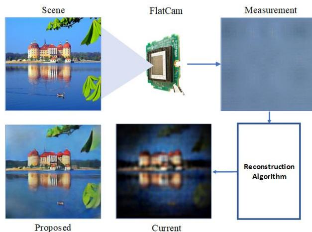
Figure 1. The FlatCam framework: The FlatCam is a thin lensless camera that captures a globally multiplexed measurement of the scene and requires a reconstruction step to recover the true scene. In this work, we propose a novel reconstruction algorithm that gives higher resolution images with improved dynamic range and robustness to noise than current methods.
