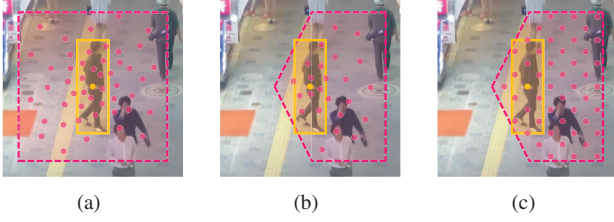
Figure 9. Comparison of sampled search points, depicted by red dots, in (a) MDNet, (b) MDNet+FM, and (c) CDT+FM. The points in (a) and (b) are sampled from a Gaussian distribution, while those in (c) are from a uniform distribution.
