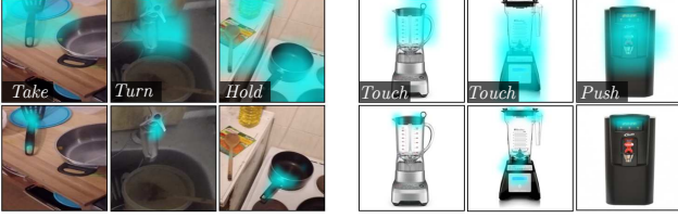
Figure 3: Our method (bottom) vs. traditional action recognition+Grad-CAM (top). Our model generates localized and affordance-relevant activations.
