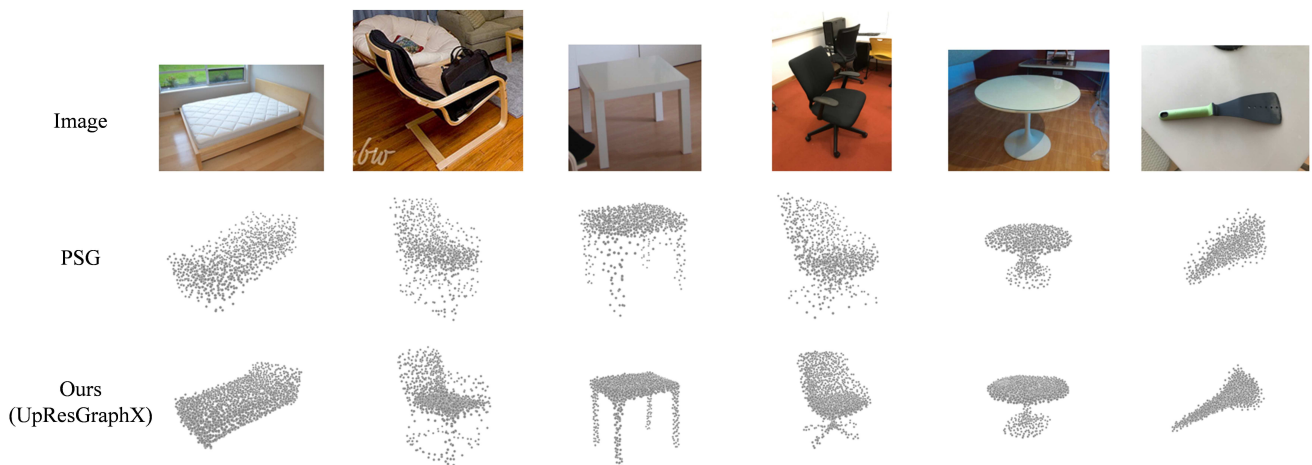
Figure 5. Qualitative performance of PSG [4] and PCDNet-UpResGraphX on some real life images taken from Pix3D. The predictions from PSG have high variance compared to ours, which present clear and solid shapes.
