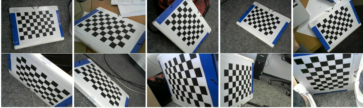
Figure 7. Sample images used for the calibration in real-world tests. Top row: freely-taken images. Bottom row: wizard guided images.
