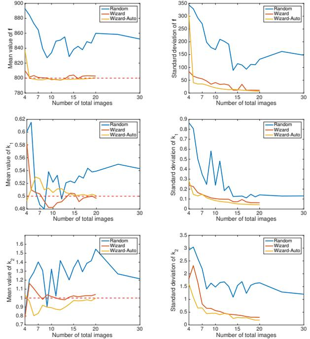
Figure 4. Comparisons of the intrinsic parameters estimated from three schemes on synthetic data: randomly taken images, calibration wizard without and with autocorrelation matrix.  $f = 800$ ,  $(u, v) = (320, 240)$ ,  $k_1 = 0.5$ ,  $k_2 = 1$ . Wizard images achieve superior performance over random images on all intrinsic parameters. Considering the autocorrelation matrices can further provide the most accurate and precise estimation outcomes.
