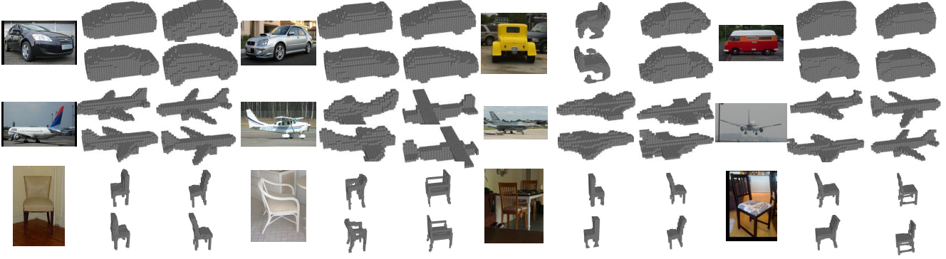
Figure 4: 3D reconstruction from single image on PASCAL 3D+. For each image, we show the predicted and ground-truth (left) voxel representation (right). We show two different views for each 3D representation.
