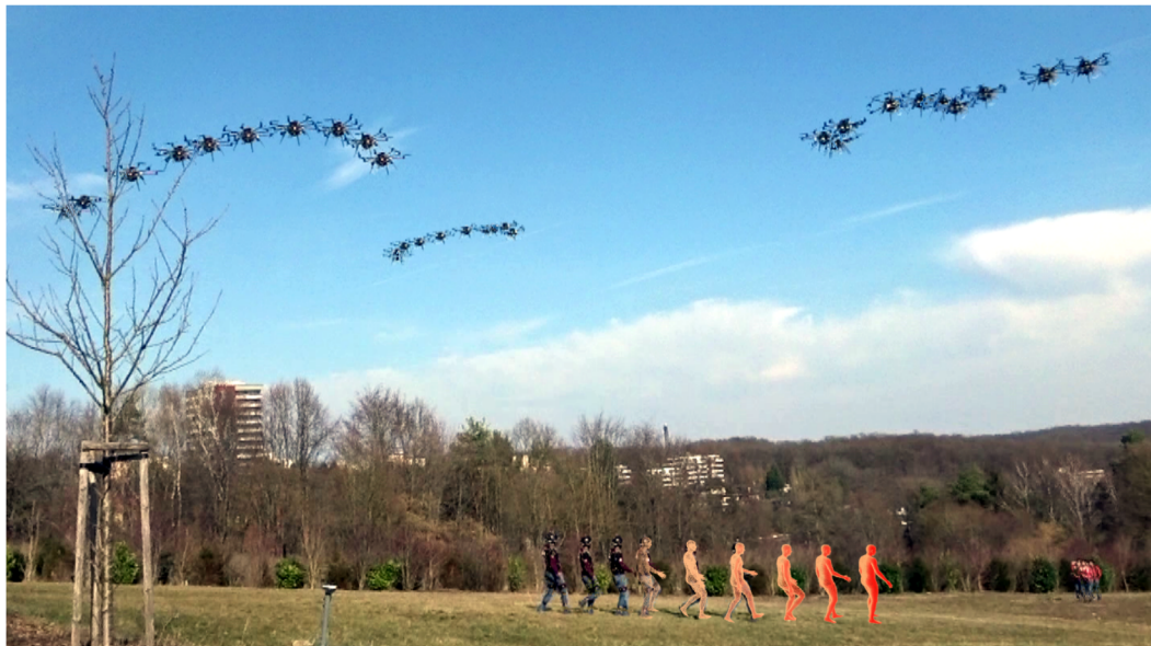
Figure 1: 3D markerless motion capture from fully autonomous micro aerial vehicles (MAVs) with on-board cameras. Multi-exposure image shows the trajectory of the MAVs and the 3D body pose and shape projected onto an image frame from an external camera. This camera was not part of the motion capture setup. Hence this camera, the MAV's cameras, body pose reprojection and alignment were manually time synchronized.
