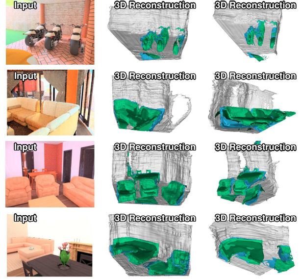
Figure 5: Single image scene reconstruction via multi-layer depth maps. Estimates of the front (green) and back (cyan) surfaces of objects, as seen from the input view, are complemented by heights estimated by a virtual overhead camera (dark green) via our epipolar feature transform. Room envelope estimates are rendered in gray.
