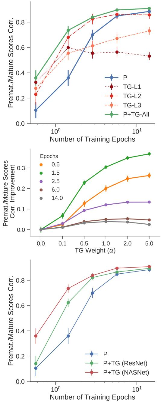
Figure 1. (top) Comparison of single layer and combined RDMs with premature performance as predictors of mature performance on NASNet. P+TG was computed using  $\alpha = 5$ . (middle) Gain in predicting the mature performance with varying TG weight. (bottom) Comparison of combined RDM scores using two alternative teacher models at various stages of training.  $\alpha$  values of 1 and 5 were used for ResNet and NASNet respectively.
