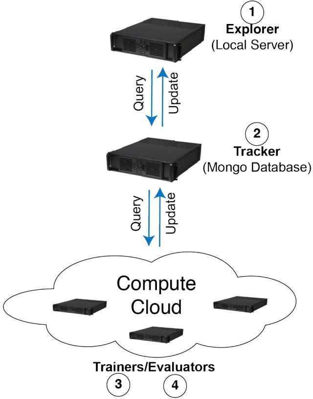
Figure 4. Implementation of a distributed framework for conducting architecture search.
