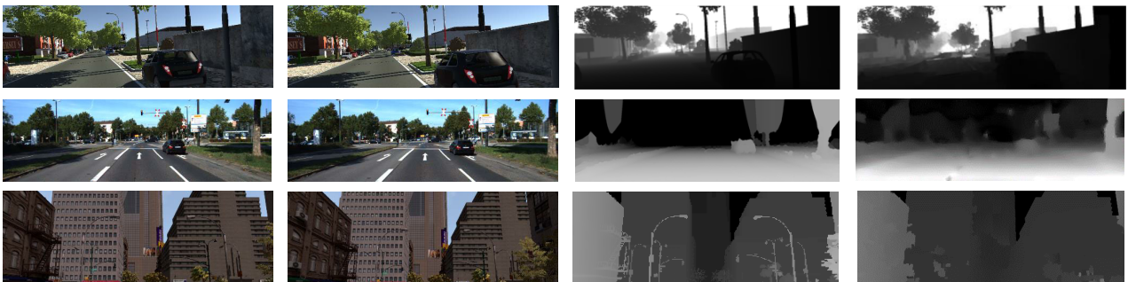
Figure 5. Demonstration of depth map estimated by Ours+CPM (T) in traffic scenes. From left to right: reference frame I_t , next frame I_{t+1} , ground truth depth map and the result of Ours+CPM (T).
