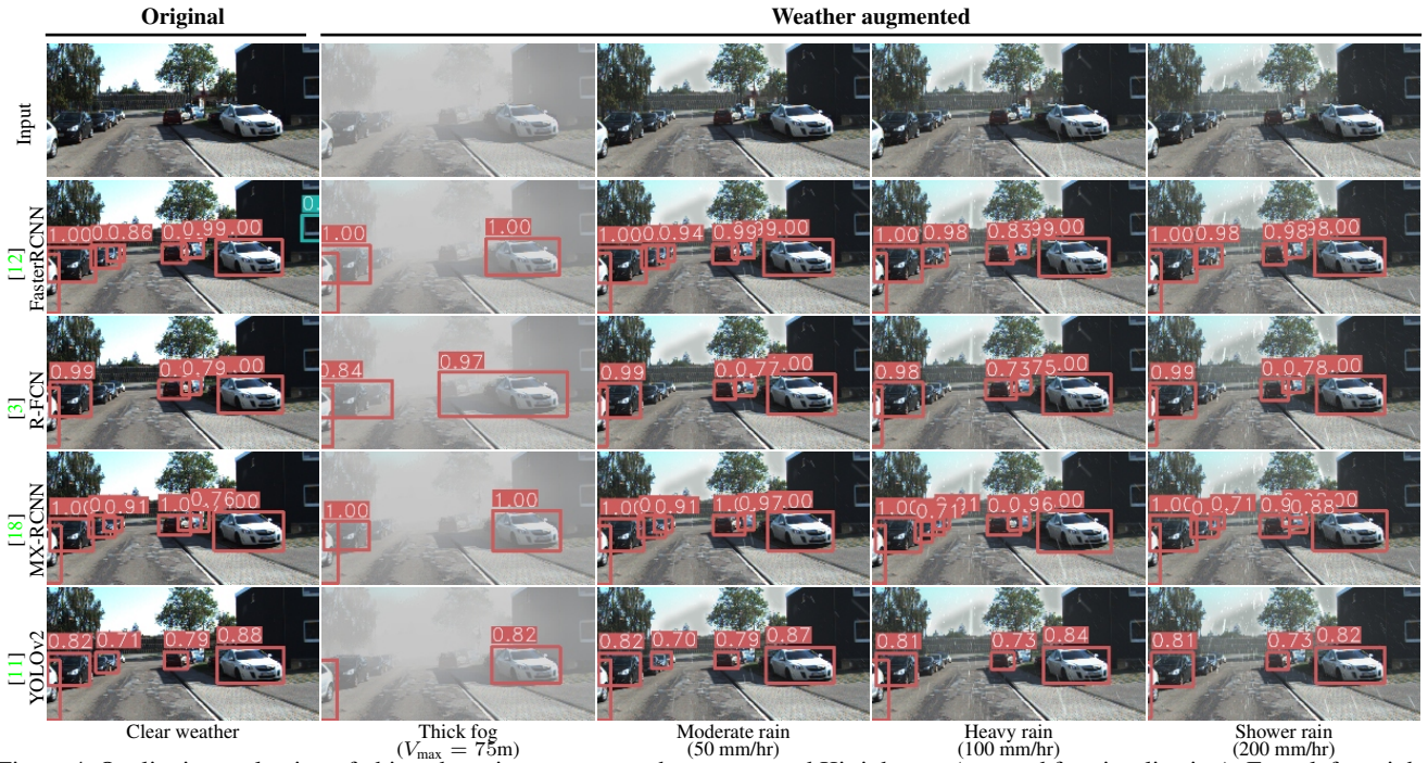
Figure 4. Qualitative evaluation of object detection on our weather augmented Kitti dataset (cropped for visualization). From left to right, the original image (clear) and four weather augmented images. In addition to a gradual decrease in the confidence of the bounding box when thresholded, the number of objects detected using R-FCN [3] or Faster R-CNN [12] subsequently decrease with rain. This behaviour is especially visible in the fog and 100+ mm/hr rain of both the set of images. With heavy rain YOLOv2 [11] output confidence of bounding boxes around objects decrease and faraway objects are not detected. Only detections with confidence \geq 0.7 are shown.
