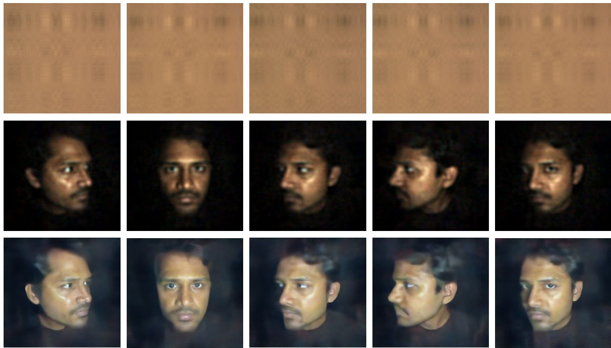
Figure 5. Reconstruction of video frames. Top row shows the captured measurement, while the second and third row show the Tikhonov regularized reconstruction and proposed reconstruction respectively.
