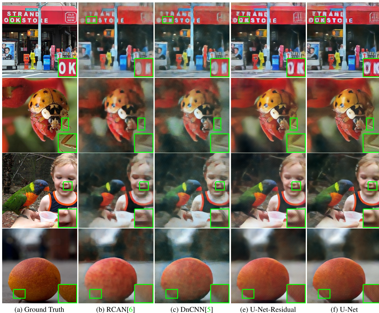
Figure 3. Comparison for display captured measurements. RCAN[6] and DnCNN[5] are unable to restore finer details such as the text in top row. U-Net-Residual is outperformed by U-Net used in the proposed architecture in restoring these fine details.
