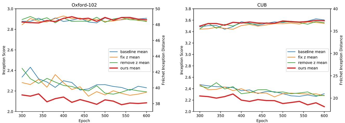
Figure 9: Inception score (left axis, top curves) and FID (right axis, bottom curves) for the baseline method, its variants (fix  $z$  and remove  $z$ ) and our method on Oxford-102 (left) and CUB (right) datasets. Each curve is the mean of three independent experiments. Higher inception score and lower FID mean better performance.
