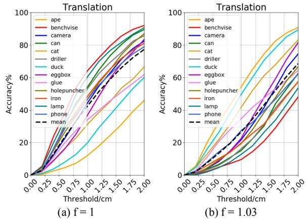
Figure 1: (a) Translation solved from coordinates without scaling. (b) Translation solved from  $f \cdot$  coordinates, where  $f$  is a coefficient to compensate the scale error. The results indicate that the unbalanced translation performance is caused by the scale error of coordinates.
