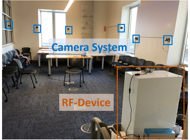
Figure 1: The figure shows our data collection system. Orange box is our radio device to collect RF signals. Blue boxes show the camera system to collect video frames. RF signals and video frames are synchronized.
