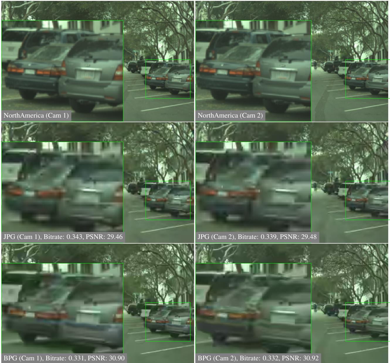
Figure 8: Comparison between the reconstructions of competing baselines and our method on a NorthAmerica stereo pair. We observe that our method yields the highest PSNR at the lowest bitrate compared to all competing methods (34% reduction in residual bitrate compared to Ballé).
