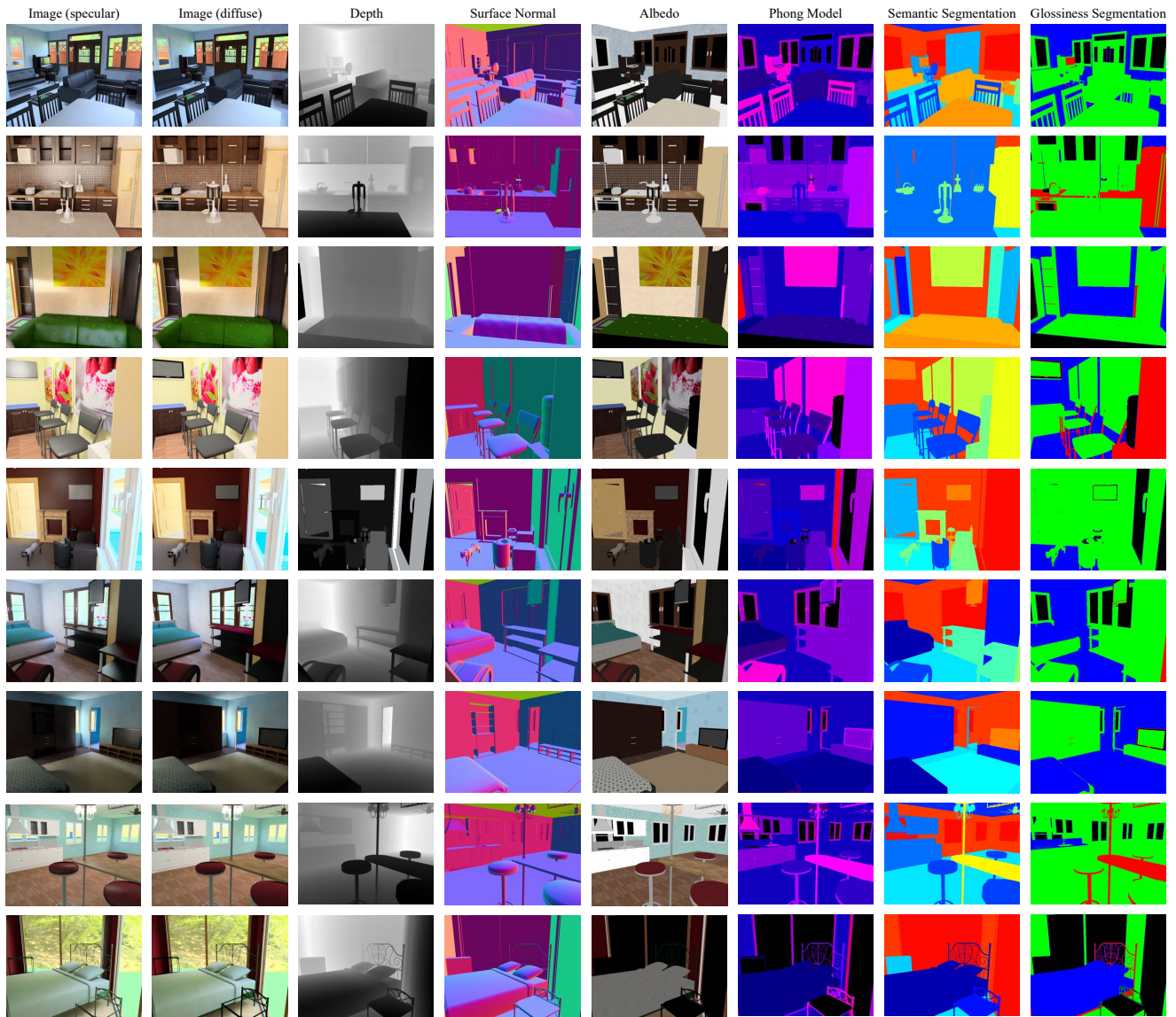
Figure 3: Our CG-PBR Dataset consists of 235,893 images of a scene assuming specular and diffuse reflectance along with ground truth depth, surface normals, albedo, Phong model parameters, semantic segmentation and glossiness segmentation.
