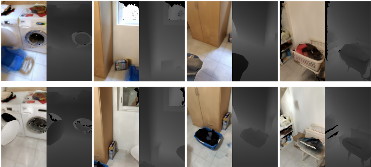
Figure 7: Example 2D projections of the color and depth of two corresponding reconstructions with natural scene changes.
